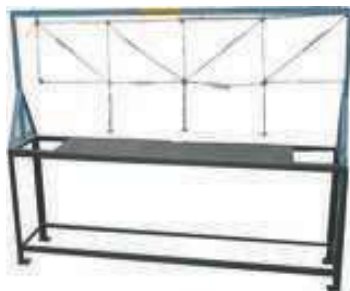
DEFLECTION OF TRUSS APP.
